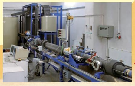
**TEST EQUIPMENT OF FLOW METERS** FOR DIMENSIONS DN 25 ÷ DN 200
