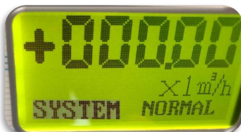
System Normal – (flow meter systems are working properly. If not, Error messages in Alarm)
