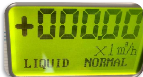
Liquid normal (measured medium is a liquid that the flow meter can measure)
